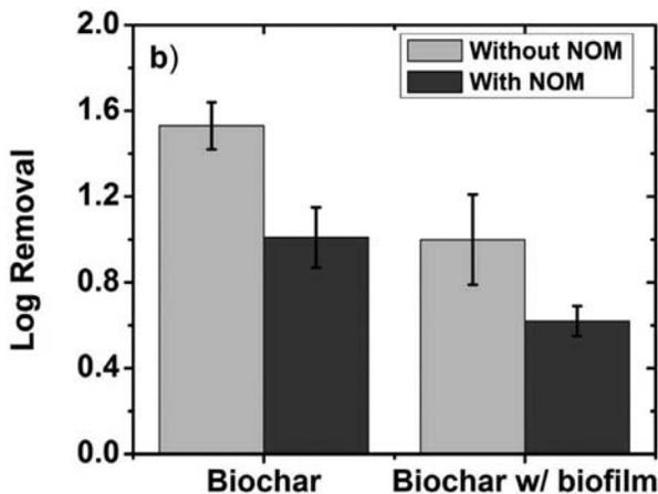
**Fig. 9** Log removal of *E. coli* in laboratorial sand-biochar (70% sand, 30% biochar: by volume) columns in presence or absence of biofilm and natural organic matter (NOM). Reprinted from Afrooz ARMN, Boehm AB, *Escherichia coli* removal in biochar-modified biofilters: effects of biofilm, *PLoS One* 11(12), open-access, © 2016 Afrooz, Boehm.
