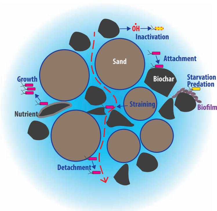
**Fig. 3** Mechanisms related to the fate of pathogens in biochar-amended filter media: straining, attachment, detachment, growth, inactivation, predation, and biofilm development.
