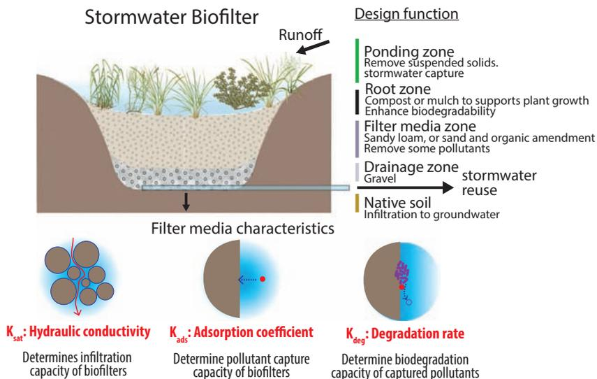
**Fig. 1** Schematic of a traditional stormwater biofilter and functions of different components of biofilters and the filter media. *Reprinted and adapted from Mohanty SK, Valenca R, Berger AW, Yu IKM, Xiong X, Saunders TM, et al. Plenty of room for carbon on the ground: Potential applications of biochar for stormwater treatment. Sci Total Environ, 625:1644–1658, Copyright (2018), with permission from Elsevier.*
