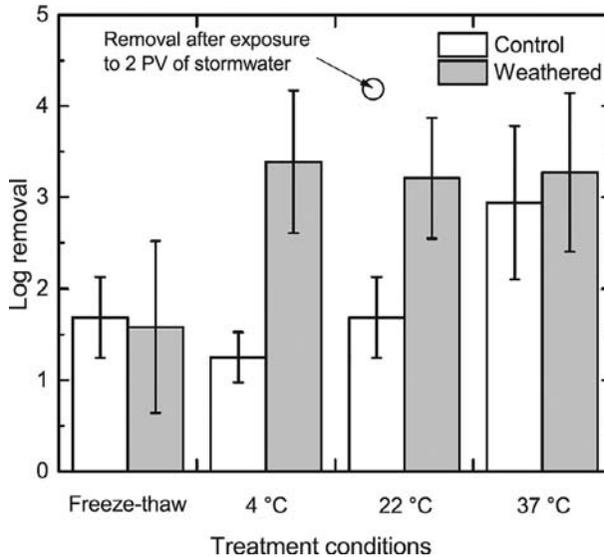
**Fig. 8** Removal of *E. coli* by sand-biochar biofilters when exposed to freeze-thaw cycles and dry-wet cycles at 4 °C, 22 °C and 37 °C. Reprinted from Mohanty SK, Boehm AB., *Effect of weathering on mobilization of biochar particles and bacterial removal in a stormwater biofilter*, *Water Research*, 85:208–215, Copyright (2015), with permission from Elsevier.
